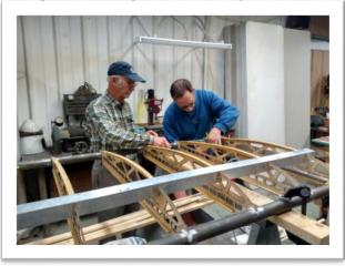
As of this writing, three wing panels are complete and the fourth wing is getting fitted with ribs as seen in the photo's. All four should be complete and ready for load-testing early 2017.
