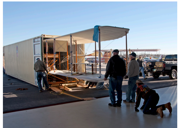
This 2013 photo of the non-flying Valentine Flyer shows how the new Wright "B" Flyer lookalike will fit into a standard shipping container. (Photo: Timothy R. Gaffney)
