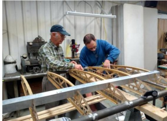
As of this writing, three wing panels are complete and the fourth wing is getting fitted with ribs as seen in the photo's. All four should be complete and ready for load-testing early 2017.
